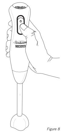
**Note:** The StickMaster<sup>®</sup> Cordless Stick Blender is designed to operate only when the power button remains pulled downwards.
